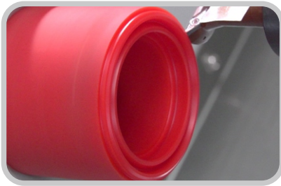
Turning sealing profiles with professional cutting edge
