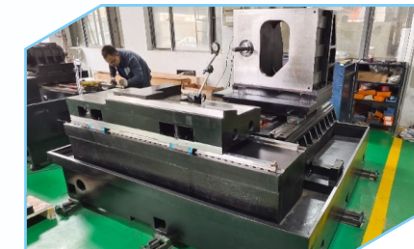
Machine base and bed adopt mixed mineral
