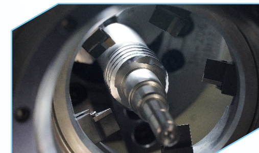
Surface roughness Ra 0.4-1.0um after milling
