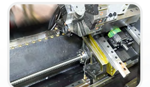
Large diameter high-speed silent ball screw, and roller guide way.
