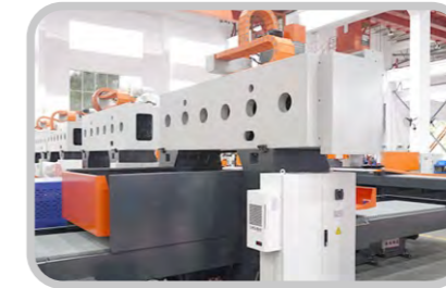
Gantry fixed beam structure
