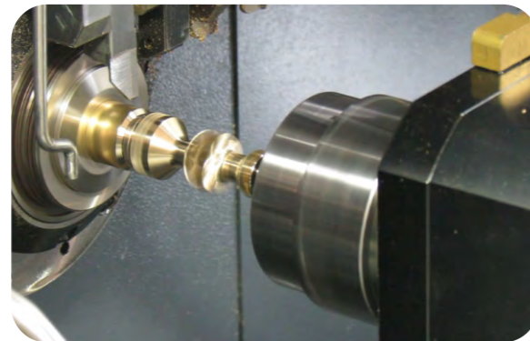
Sub-spindle butt joint workpiece with main spindle.
