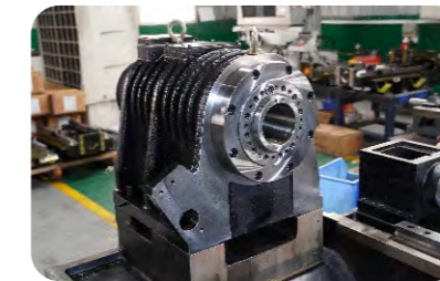
Large torque with belt type spindle
