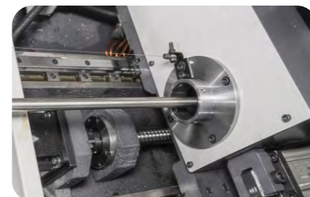
Sliding headstock move on Z axis
