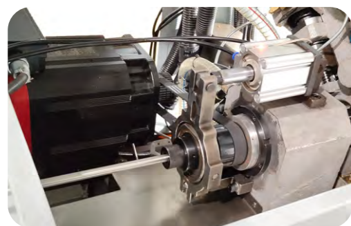
The spindle box is fixed and tool saddle can move 120mm on Z axis
