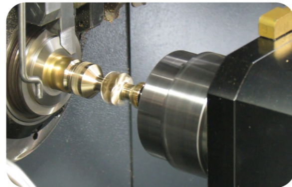
Sub-spindle butt joint workpiece with main spindle.
