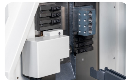
2pcs live tool on Y axis 6pcs turning tool 4pcs front drilling tool
