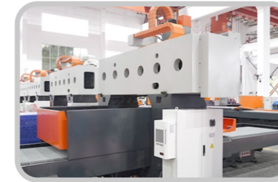
Gantry fixed beam structure
