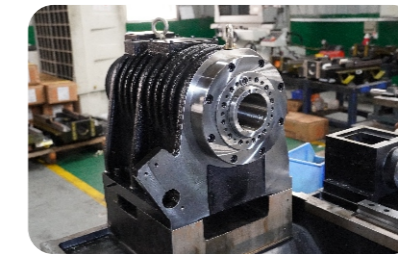
Large torque with belt type spindle
