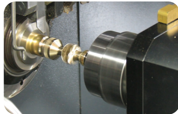
Sub-spindle butt joint workpiece with main spindle.
