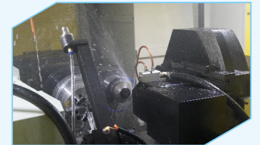
X axis and Z axis will interpolation dressing together.
